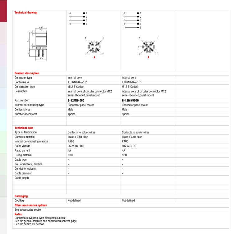
Internal cores - B-coded
