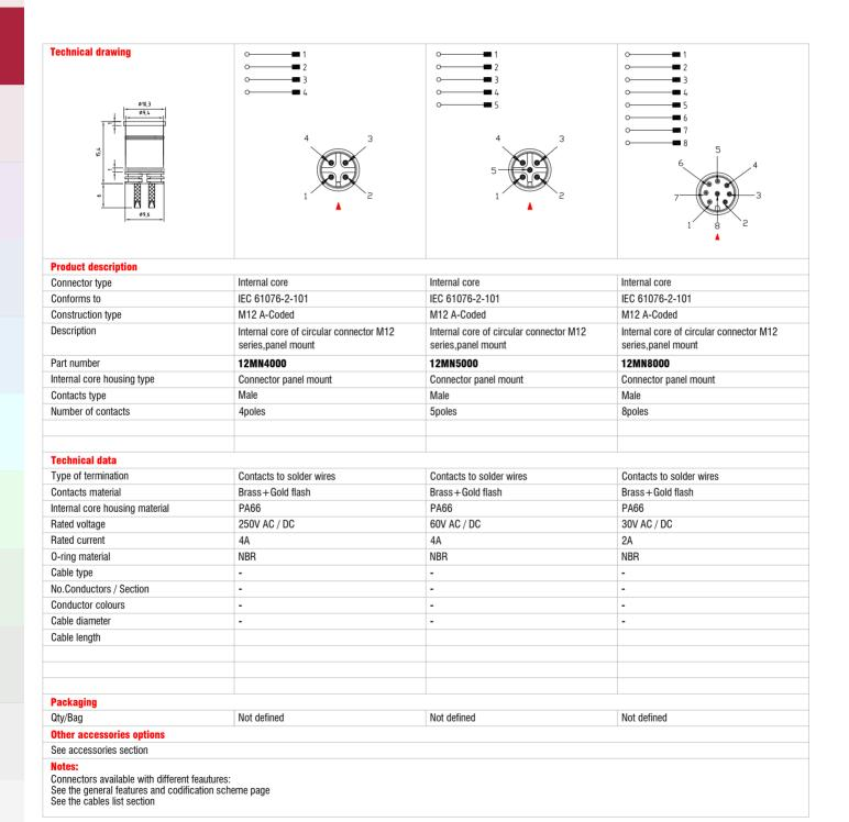
Internal cores - A-coded
