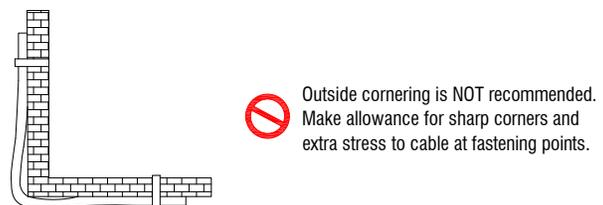
**INSTALLATION OF CABLE FOR MOTION APPLICATIONS:**
